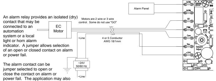
need to monitor alarm wiring integrity. An open on alarm or power fail configuration provides some level of line failure protection since an open wire will also create an alarm. Some alarm panels can be configured to monitor an EOLR (end of the line resistor). Place the wiring EOLR across the ALRM connections and Jumper select open on alarm or power fail.
